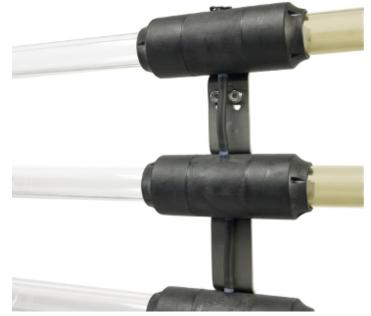
UV lamps in TrojanUV systems are enclosed in a quartz sleeve to insulate them from the water. ActiClean<sup>™</sup> is our patented dual-action sleeve cleaning system that uses mechanical wiping in conjunction with ActiClean Gel contained within wiper canisters surrounding the quartz sleeves.
