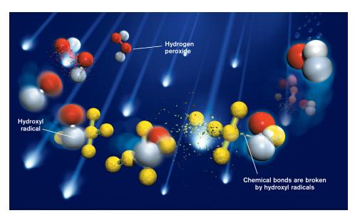
UV light in combination with hydrogen peroxide creates hydroxyl radicals that break the bonds of chemical contaminants, reducing them to their safe, elemental components.
