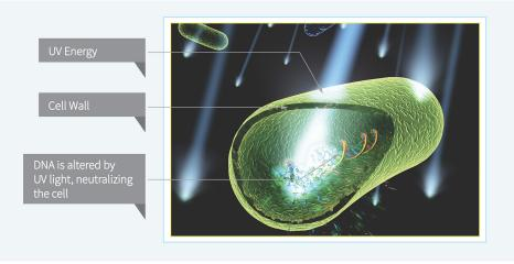
There are a few key differences between UV disinfection and chemical methods. UV does not add anything to the water except light. As such, there is no balancing act between dosing and residuals, so there is no risk of exceeding THM (trihalomethanes) limits or chlorine residual requirements.
